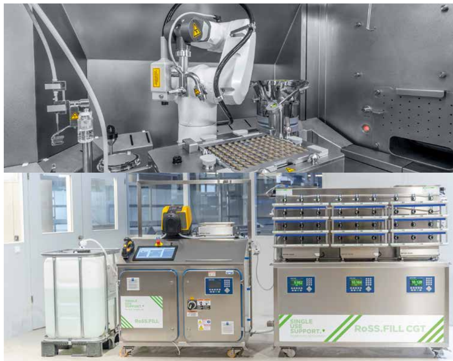
Figure 6 - Crystal® L1 robotic vial fill line (top) and Single Use Support ROSS.FILL CGT bag filler (bottom)
